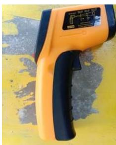
**Gambar 11.** Termometer Infrared
