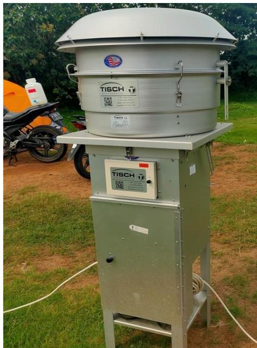
Gambar 1. *High Volume Air Sampler (HVAS)*
