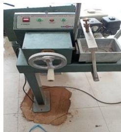
Gambar 4. Direct shear test
