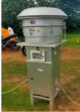
**Gambar 1.** *High Volume Air Sampler* (HVAS)
