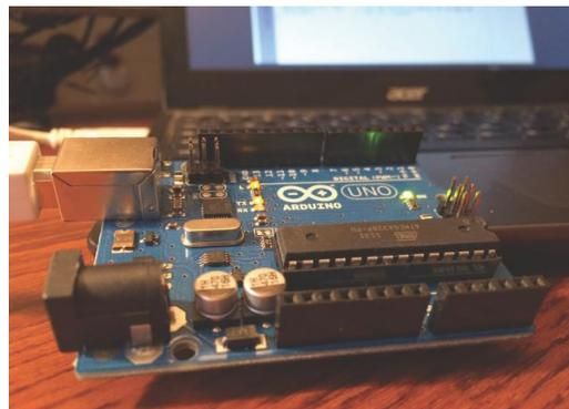
Gambar 3. Papan ARDUINO
