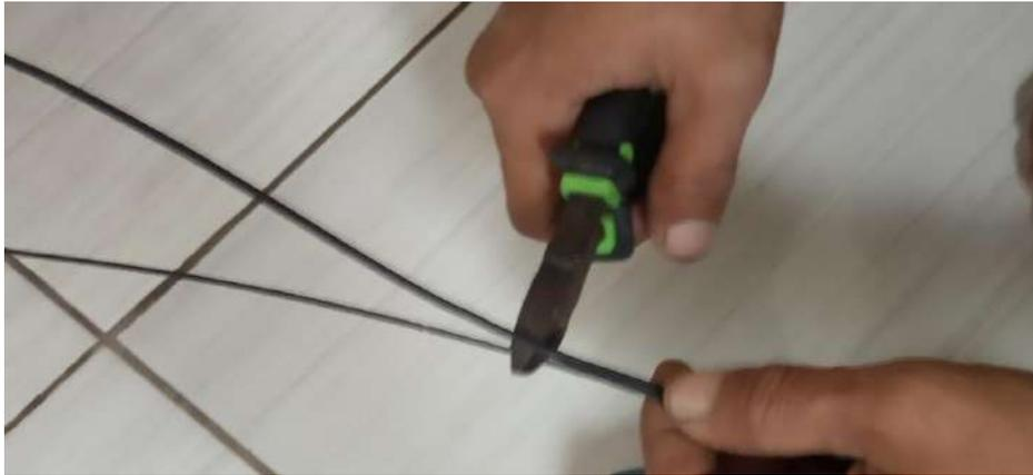
**Gambar 7.** Memotong sling
